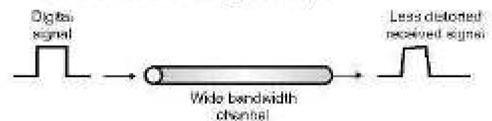
(a) Baseband transmission through a wideband channel
