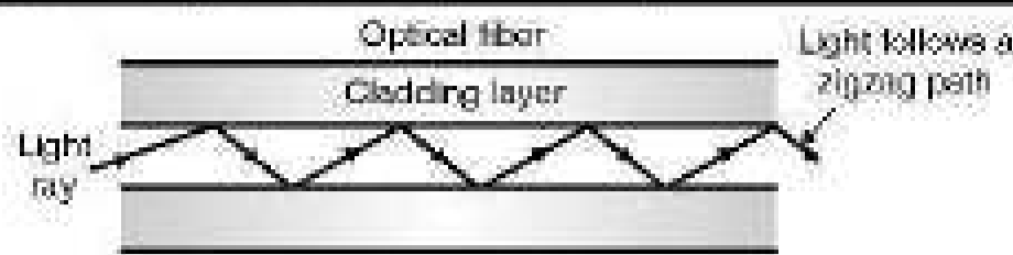
(a) Light follows a zigzag path within the optical fiber
