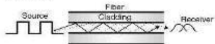
(8-111) Fig. 3.4.7 : Light propagation in multimode step index fiber
