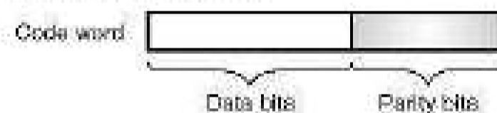
(L-303) Fig. 6.1.5 : Structure of a transmitted code word
