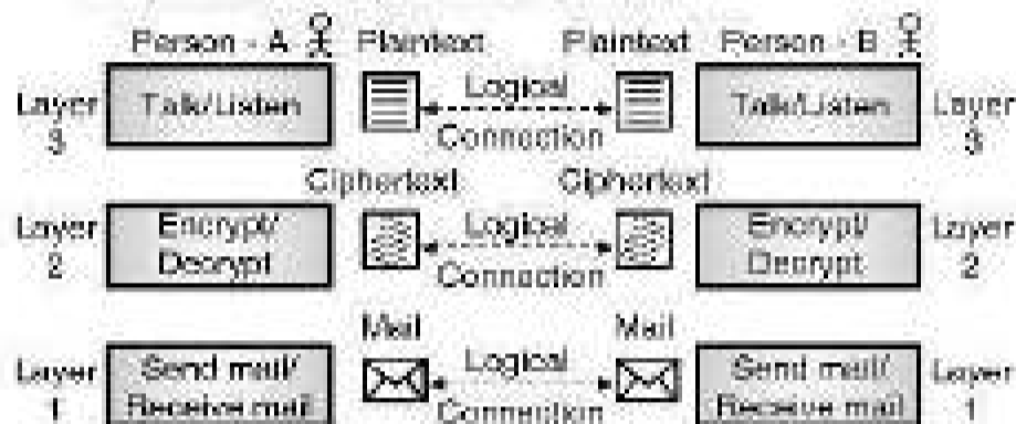
(G-2064) Fig. 11.2.2 : Concept of logical connections between the peer layers
