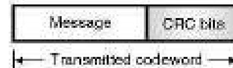
(L-912) Fig. 6.4.1 : Structure of transmitted codeword using CRC
